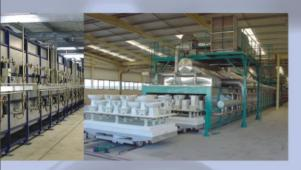
The tunnel kiln is a flexible and innovative production aggregate in prefabricated modular design with refractory lightweight brick or fibre lining, equipped with latest kiln control systems and kiln car tracking systems, for different fields of application and firing of:
